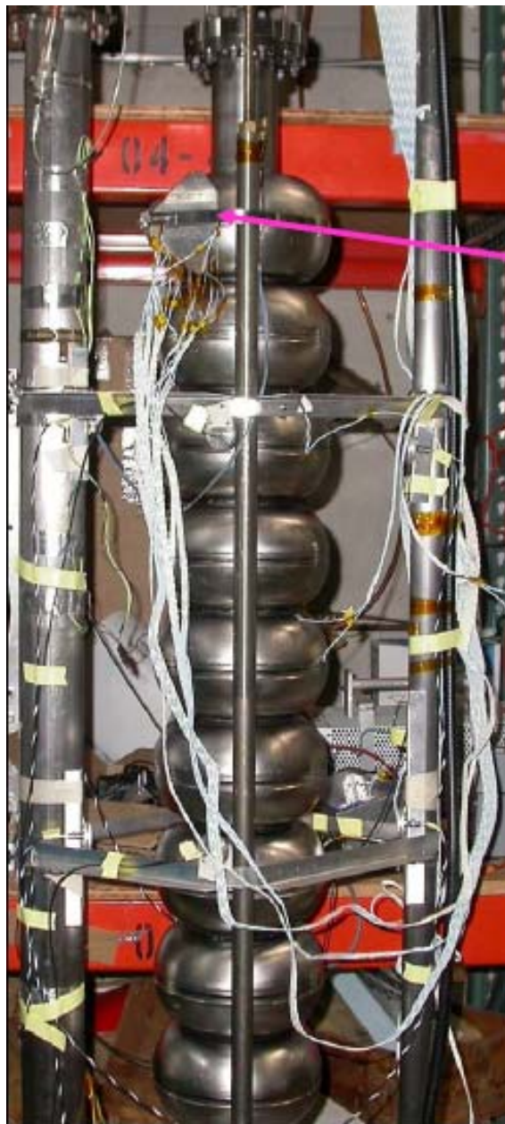
Figure 4.5.: TESLA cavity at Cornell, the arrow indicates the quench location. [7]
