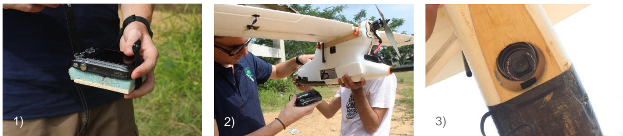
Figure 3. 1) Camera embedded on sponge; 2) Mounting the camera into the fuselage; 3) Camera hole at UAV bottom
