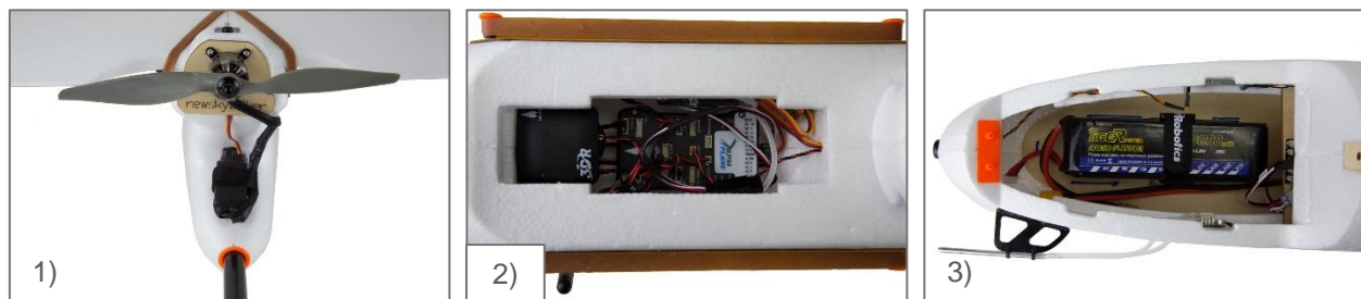
Figure 2. 1) Motor and propeller; 2) Pixhawk autopilot; 3) LiPo battery
