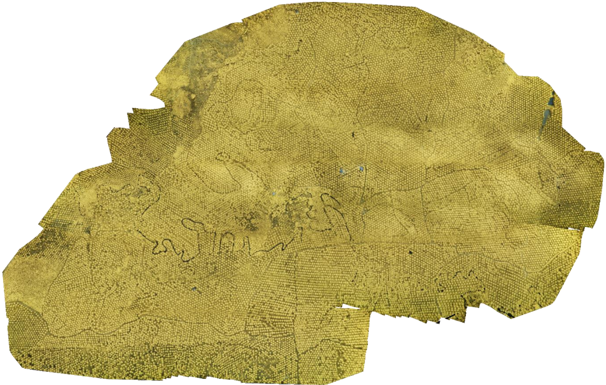
Figure 24. Orthorectified photomosaic of the research area, with NIR, green and blue color channels
